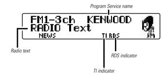
Description about this indicator for these features can be displayed by setting the Lower Part Display (page 12) to "... + Function indicator"
